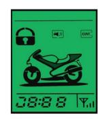
moved, the alarm will chirp and the indicator will flash lights 5 times, LCD remote fob hammer icon will flash and vibrate. If it's moved hard after 10 seconds then full reaction will occur and sound for 30 seconds. Engine will be completely immobilised and can not be driven away.
