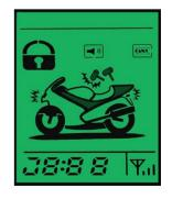
During 2<sup>nd</sup> stage (full alarm mode) if alarm is triggered within 10 seconds after 1st stage. Then system will go into full alarm mode. Siren will activate for 30 seconds and indicator lights flash for 30 seconds and engine will be immobilise.
