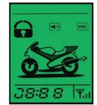
and used for non-key driving and warm-up. Repeat the above operation if the engine does not function due to cold weather or due to slow rotation of engine. Engine will stay on 10 minutes.
